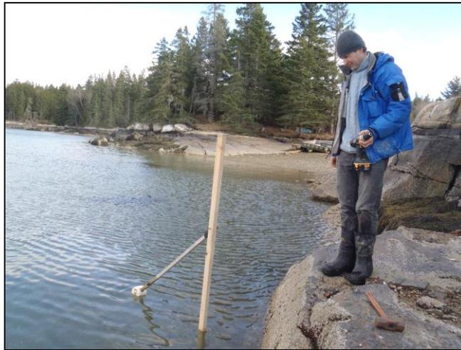
Above, Vitalii Sheremet admires newly installed pivot tide gauge that measures low tide level inside lobster pound at Friendship Long Island. Photo by Diane Cowan. Arrow at right, PVC pipe attached to piling serves as enclosure for reel tide gauge. Photo by Vitalii Sheremet.
